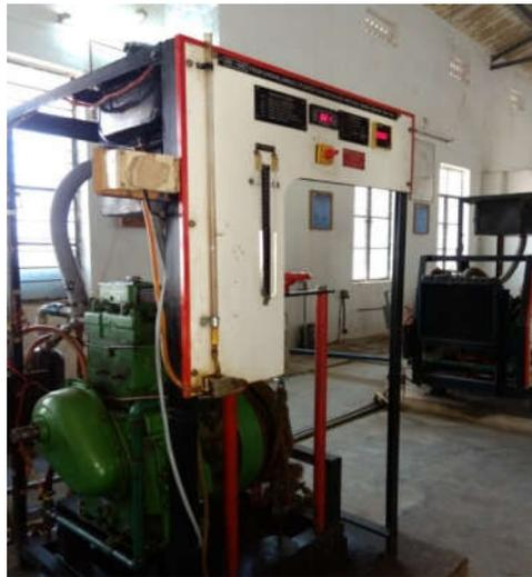
Figure 1. Single-cylinder 4-stroke diesel engine.
