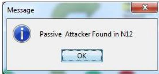
From the above window we can clearly identify there is one intrusion attack found in Node N12 and this is identified dynamically by the end user and the same router immediately try to regenerate a new path and send the data to the valid destination under a new dynamic path. This path will be chosen from the Node N12, but not from the starting N1 onwards.
