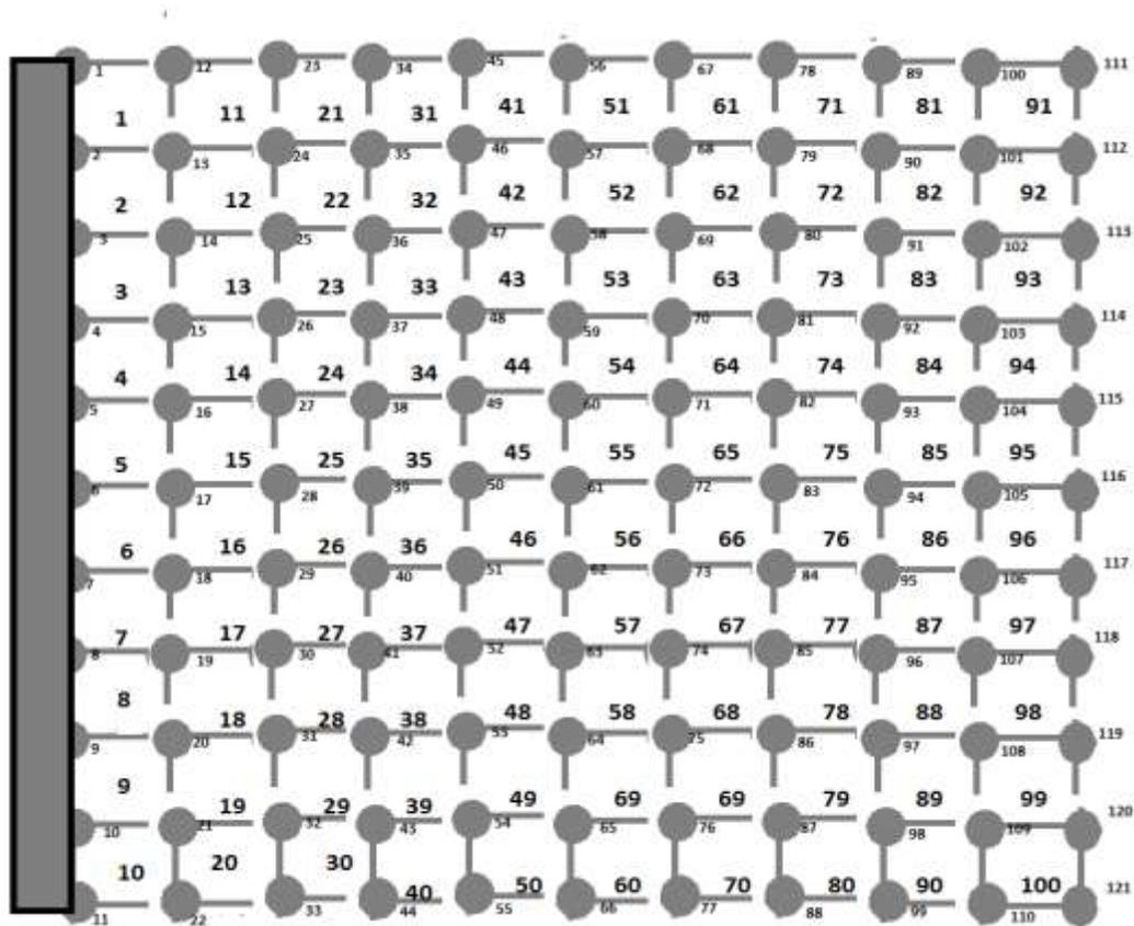
Figure 2.2: cantilever plate with 100 elements and 121 nodes
