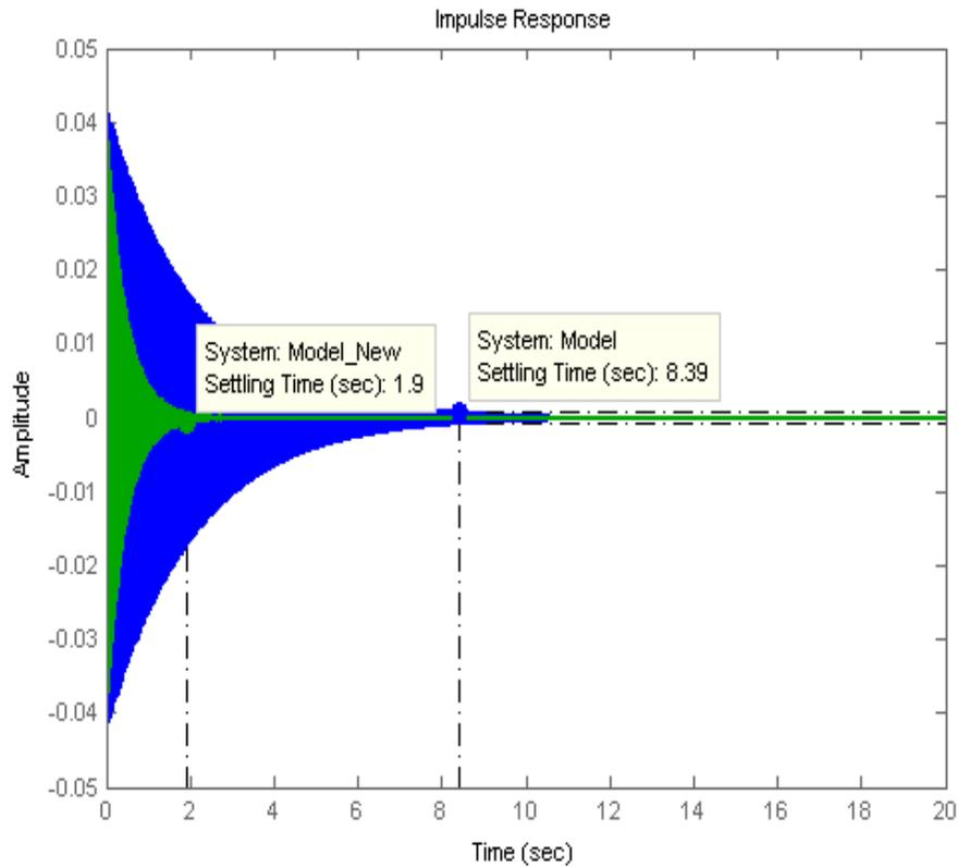
**Fig 4.1. Controlled and Uncontrolled Tip Displacement When piezoactuator is placed at 5<sup>th</sup> position (al=100 and bet=110)**
