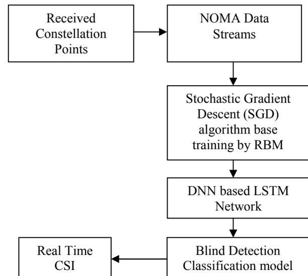
**Fig. 1: PROPOSED MODEL OF INTERFERENCE MODULATION ORDER DETECTION**
