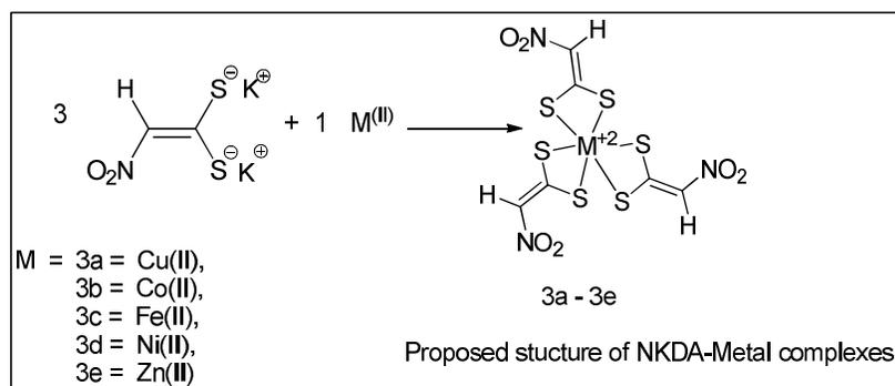
**Scheme 1: Schematic representation of synthesis of NKDA-Metal complexes**
