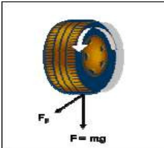
Fig. 2. Friction force  $F_\mu$  and the normal force  $F = mg$ , where  $m$  is the mass supported by the wheel and  $g$  is the acceleration of gravity  $g = 9.81$  m/s.
