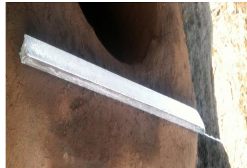
RECTANGULAR ROD AFTER CASTING
