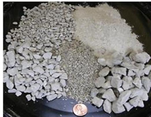
(b) RA particles with variable grain sizes
