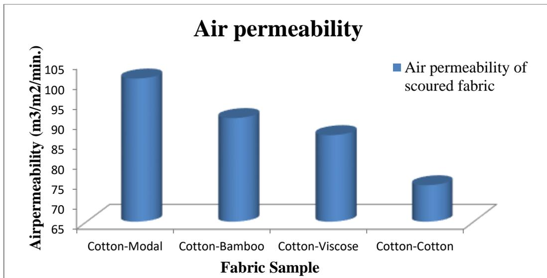
**Fig.1 Air permeability of scoured fabrics**
