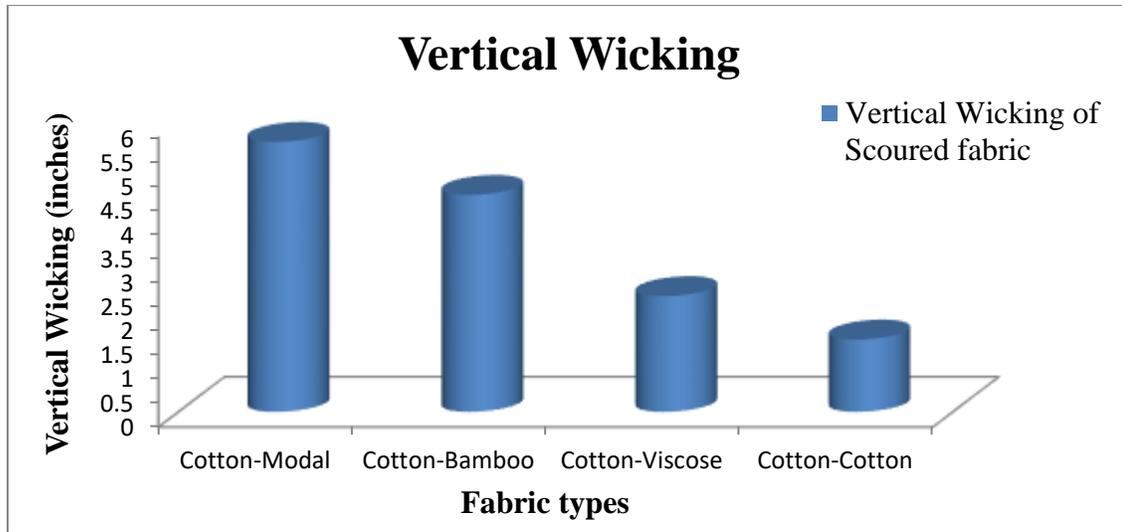
**Fig.2 Vertical Wicking of scoured fabrics**
