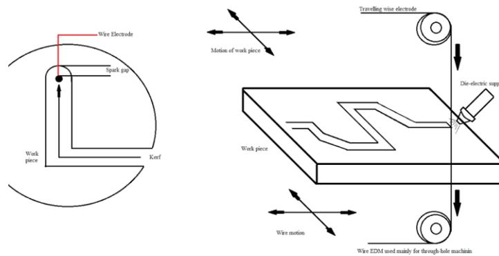
**Figure 1. Working principle of WEDM**
