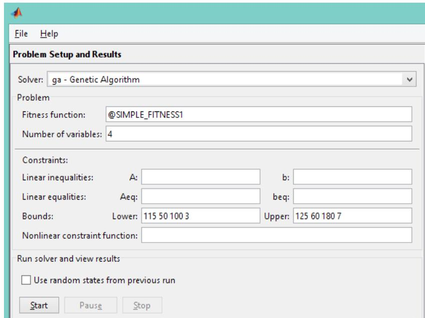
Figure 2. Input to Genetic Algorithm.
