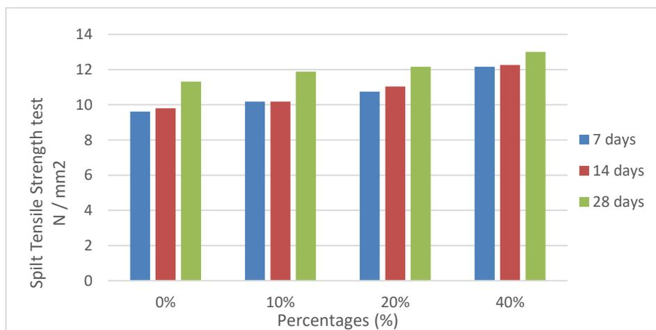
Figure 3. Graph representation of split tensile test (cylinders)
