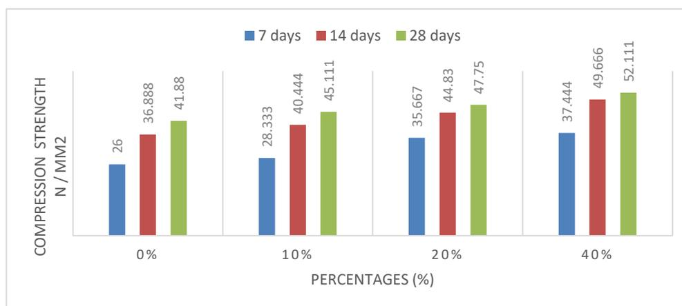
Figure 1. Graph representation of compression test (cubes)
