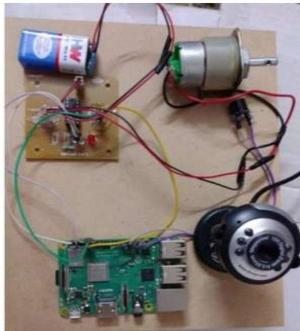
Figure 6. Hardware kit of proposed automatic gate opening system.
