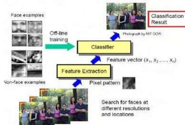
Figure 5. Block diagram of proposed face detection system.
