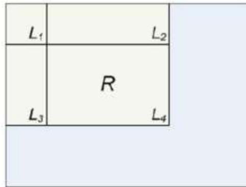
Figure 3. Calculating the area of a rectangle R is done using the corner of the rectangle:  $L4-L3-L2+L1$ .
