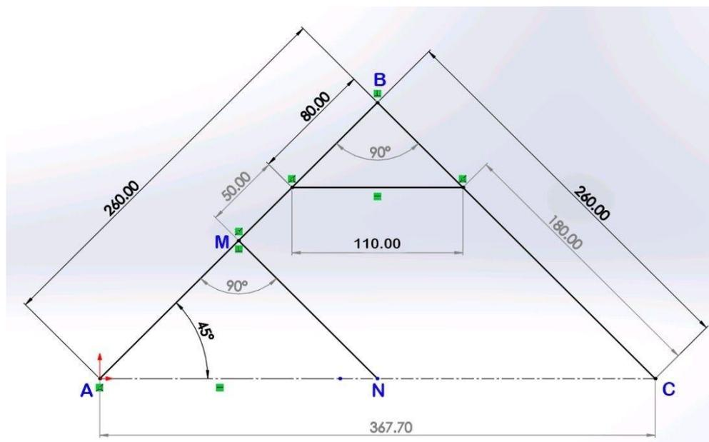
Figure-3: Design dimensions of the mechanism
