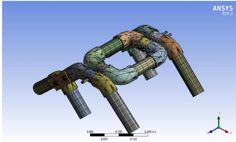
Fig-6: Image showing the meshing details of the model
