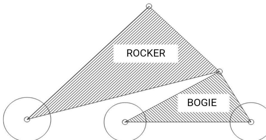
Figure-1: Kinematic diagram of Rocker-Bogie suspension
