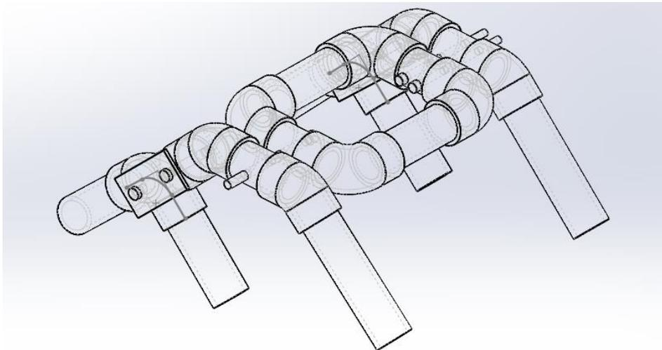
Figure-5: 3D-Model of Rocker Bogie Mechanism (Isometric)
