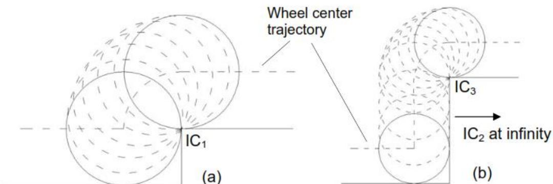
Figure-2: Wheel passing over an obstacle having (a) equal height having the radius of wheel (b) height more than the radius of wheel
