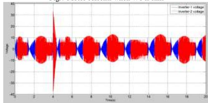
Fig.8 Inverter voltage with one leg open
