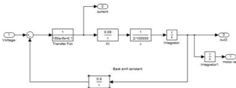
Fig.3 Mathematical model of BLDC motor
