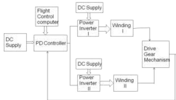
Fig.1 ElectroMechanical Actuator Block Diagram
