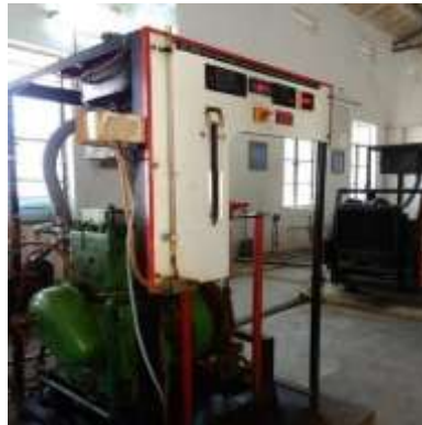
Figure 1.Single cylinder 4-stroke dieselengine.
