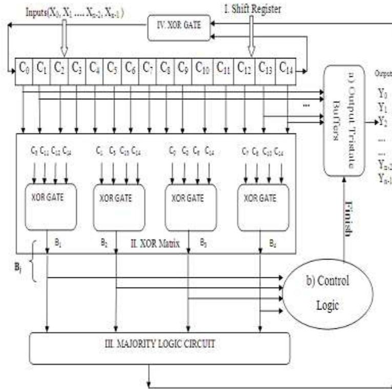
**Figure 1: Schematic of the proposed MLDD for 15 bit code word**
