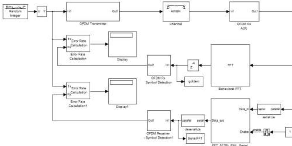
Figure1: Block diagram 512-Pt FFT processor
