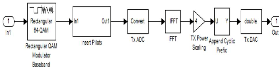
Figure2: OFDM Transmitter
