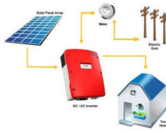
Figure 2: On-Grid Solar Panel System
