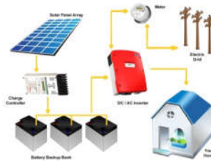
Figure 3: Hybrid Grid Solar Panel System
