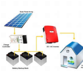
Figure 1: Off Grid Solar Power System
