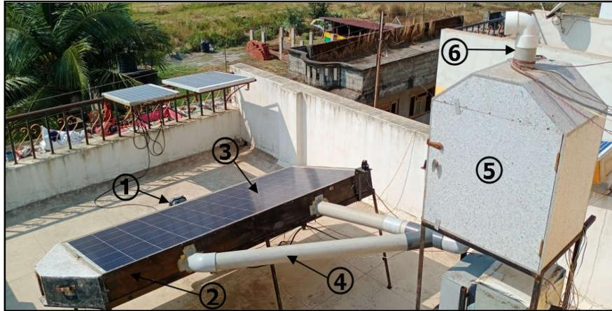
Fig 1 Experimental setup 1) 30W DC Blower 2) Enclosure 3) PV Panel as absorber 4) PVC pipe for carrying hot air 5) Drying cabinet 6) Chimney.
