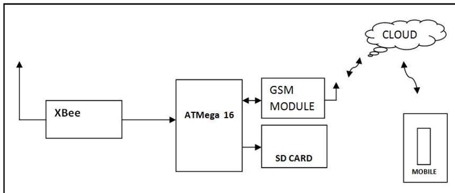
Fig 2 (b) Receiver System Architecture.
