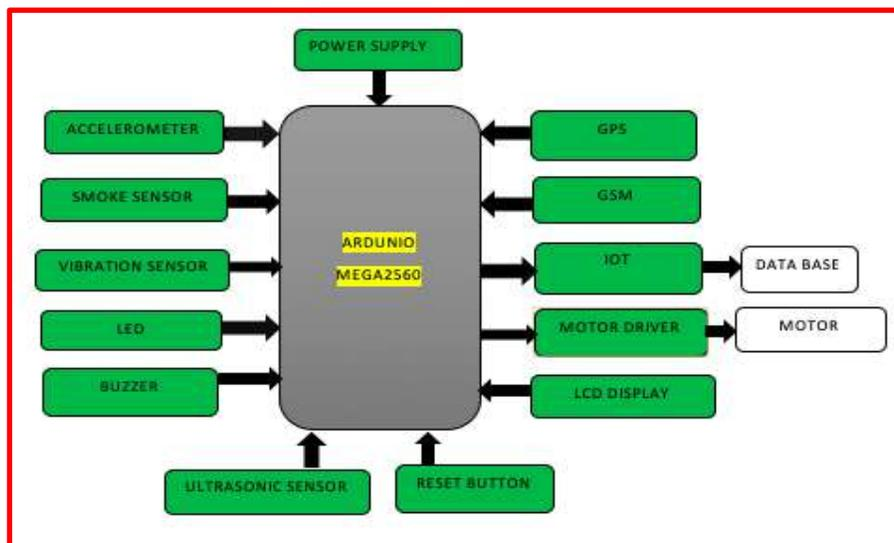
Figure 1. Block Diagram of Intelligent Accident Detection and Notification System
