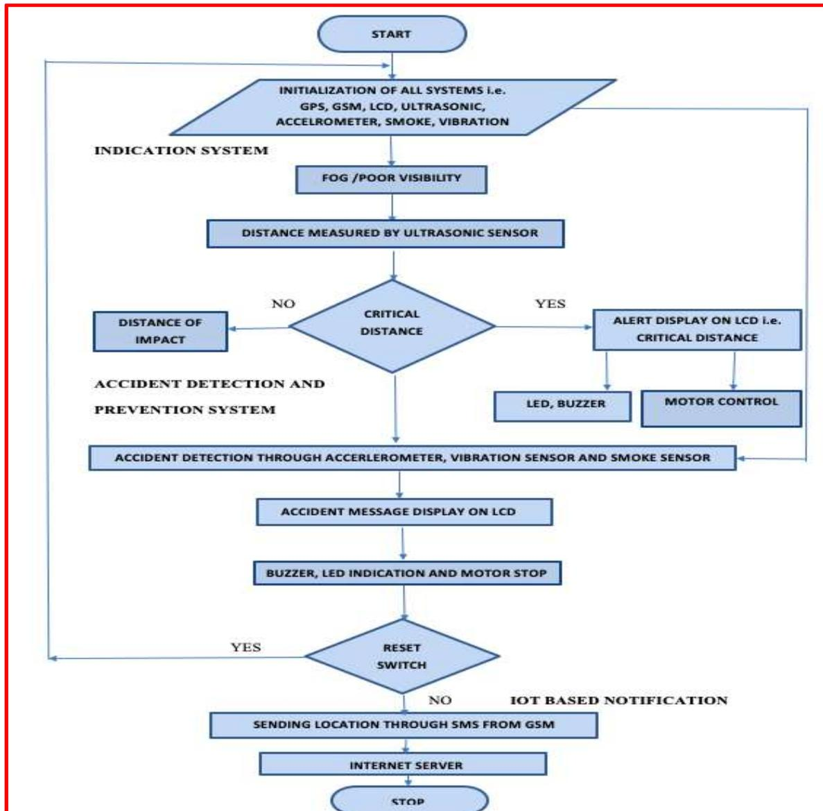
Figure 3. Flowchart of the Accident Detection & Prevention System
