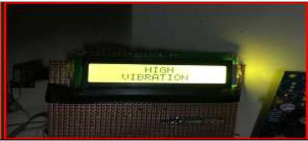
Figure 10. Vibration Sensor Detects Collision
