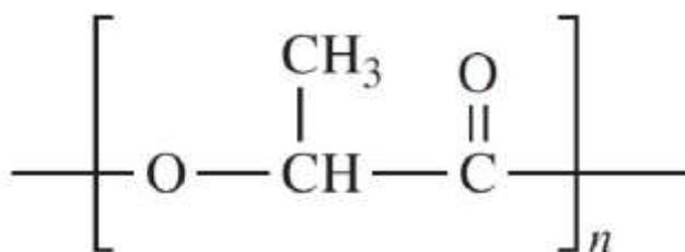
**FIG 2: Structure of Poly Lactic acid [PLA]**
