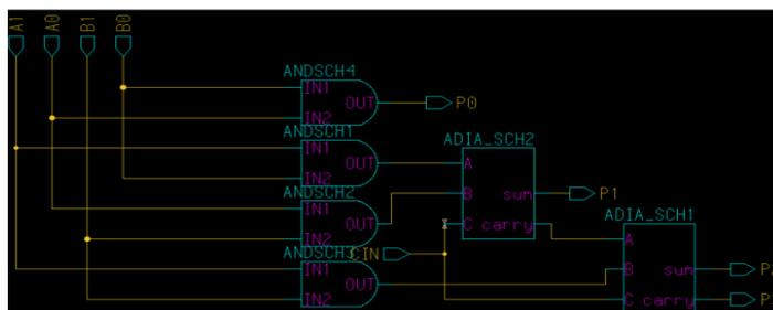
Figure 11: Multiplier 2x2 circuit
