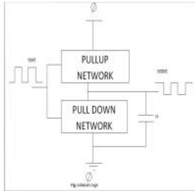
Figure 3: A Simple Adiabatic Logic Gate
