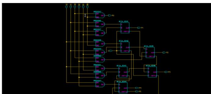
**Figure 12:**Multiplier 3x3 circuit
