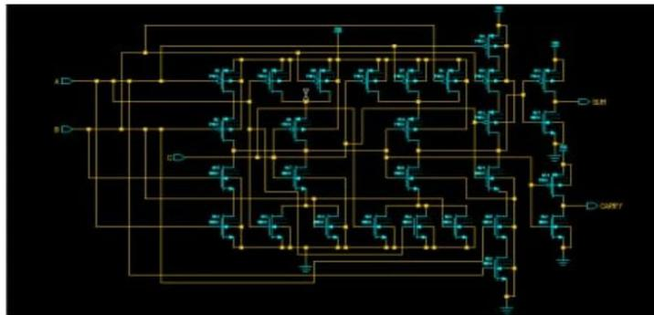
Figure 7: Basic full adder circuit(28T)
