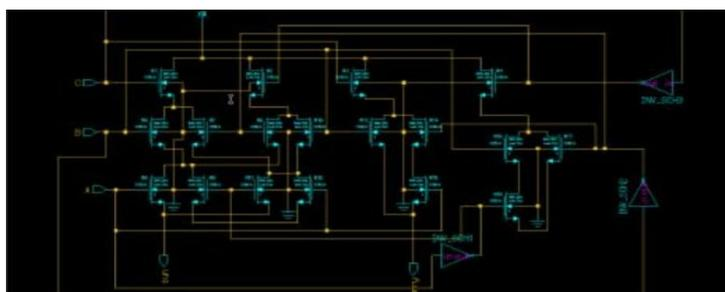
Figure 10:18T full adder circuit
