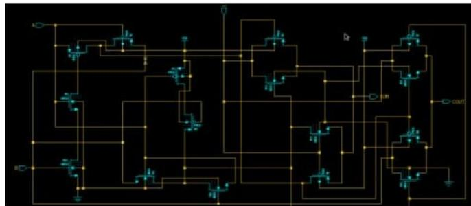
Figure 9:16T full adder circuit
