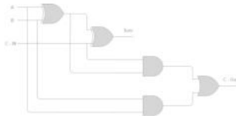
**Figure 2:** Full Adder logic circuit
