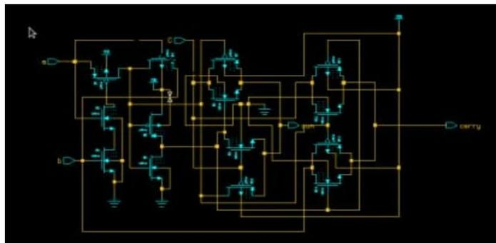
Figure 8:14T full adder circuit
