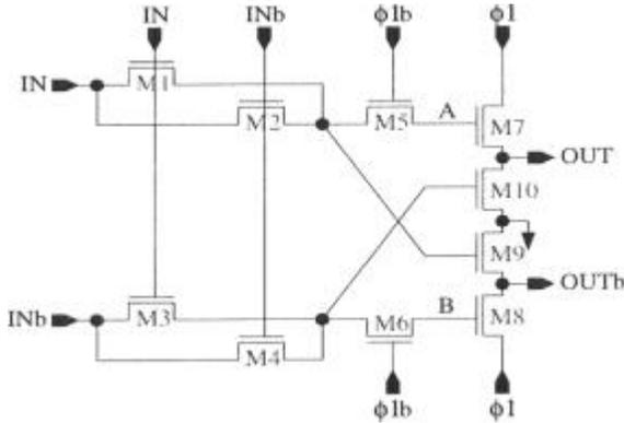
Figure 6: NMOS energy recovery logic gate
