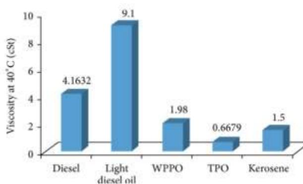
Fig. 5. Graphical comparison of viscosity different oil
