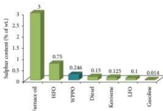
Fig. 9. The sulphur content of different types of fuel oil.
