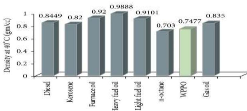
Fig. 6. Graphical representation of the density of different types of fuel
