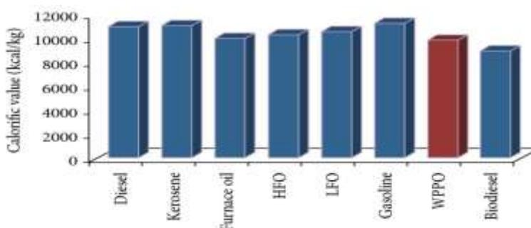
Fig. 8. Comparison chart of calorific value of oil
